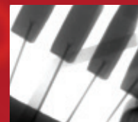
Bond Wire Inspection
