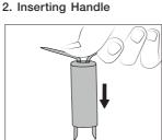
Push the grip with the tabs onto the handle.
