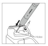
Use the holes to fix the heating element.
