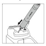
Place the handpiece on top of the new heating element and press down slightly.
