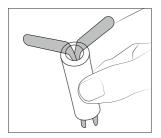
Insert the slide-on tabs into the new grip.
