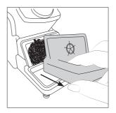
Remove the wiper by pulling it out.
