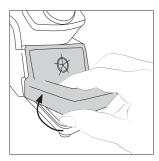
Lift the wiper at its front edge.
