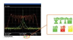
The intuitive icons help user grasp the current setting conditions all the time. As all status icons are clearly shown at the corner of the screen, there is no need to worry about the unknown settings, which may cause confusion and lead to measurement errors.
