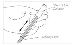
Clean the inside of the glass solder collector with the cleaning stick.
