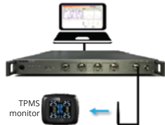
Testing a TPMS Controller with a C-1100
